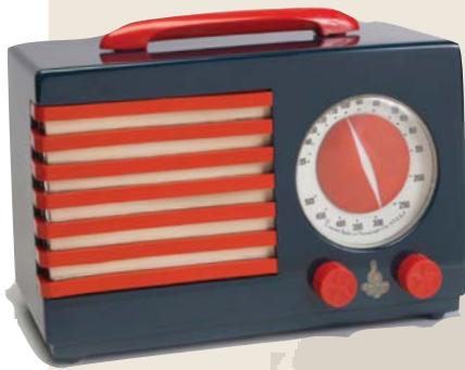
Patriot Radio, 1940, Norman Bel Geddes, manufactured by Emerson Radio and Phonograph Corp. (New York, New York), cast phenolic plastic (Catalin), molded urea plastic, molded cellulose acetate, embossed acetate, metal. Gift of George R. Kravis II, 2014, 10 1. Photo: Matt Flynn, © Smithsonian Institution.
